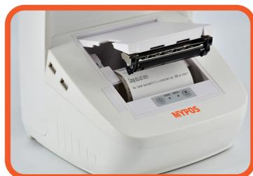
Build-in 80mm. Thermal Printer
